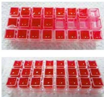
**Fig. 3.** Tightness test by means of rhodamine dye. Above: a leaking component during the test cycles, bottom: a tight component at the end of application development (© Herrmann Ultraschall)
