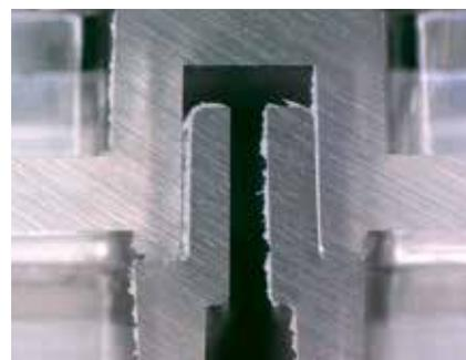
**Fig. 7.** Final assessment in the light microscope: centered homogeneous joining result (© Herrmann Ultraschall)
