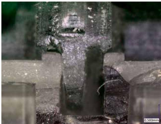
**Fig. 5.** The cut image at the beginning of the tests reveals that the component is not yet correctly centered and that further modification of the injection molding tool is required (© Herrmann Ultraschall)
