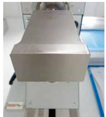
**Fig. 4.** The surface of the weld tool (sonotrode) needs to be finely polished to prevent unwanted melting (© Herrmann Ultraschall)
