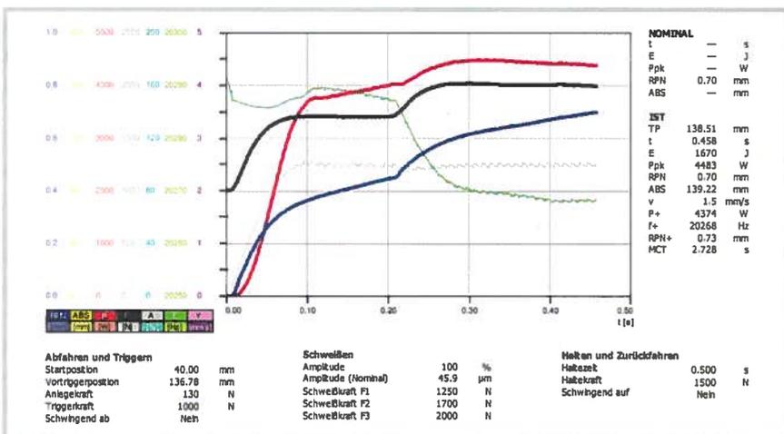
**Fig. 5.** The courses of the parameters joining distance (RPN), power (P), and force (F), as well as the correct selection of amplitude (here: 45.9 µm) and frequency (here: 20,268 Hz) are the keys to successful process settings (© Herrmann Ultraschall)
