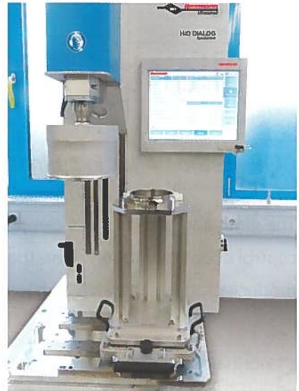
**Fig. 4.** HiQ Dialog 6200: The ultrasonic welding machine has a vertically adjustable tool holder and can display the weld course graphically on its 15-inch screen (© Herrmann Ultraschall)
