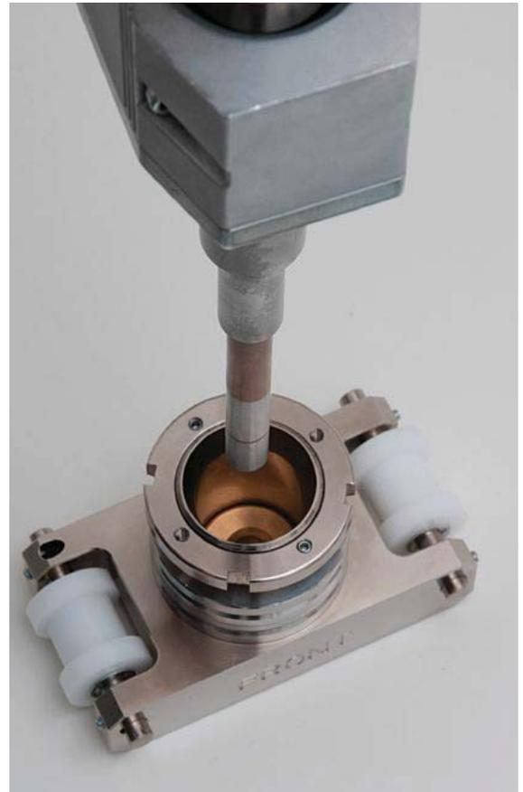
Herrmann has introduced a new ultrasonic welder that simultaneously punches out a polyester membrane from a reel of material and welds it to a plastic housing. Photo courtesy Herrmann Ultrasonics Inc.
