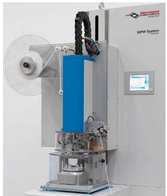
This ultrasonic welder offers five operating modes: time, energy, power, absolute distance (end point of the weld distance), and RPN distance (referencing weld depth to a starting point). Photo courtesy Herrmann Ultrasonics Inc.
