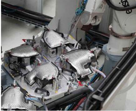
**A six-axis robot uses an ultrasonic spot-welding tool to assemble plastic insulation panels for an engine compartment. Photo courtesy Herrmann Ultrasonics Inc.**
