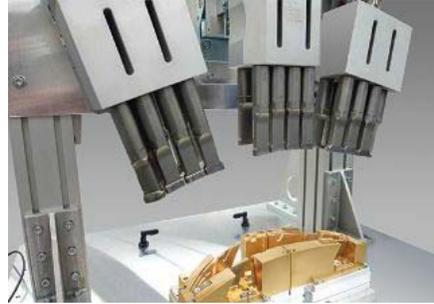
**To assemble model variants of daytime running lights, all parts of this ultrasonic welder form a “quick-change tooling frame” that can be detached from the main machine and exchanged with a different frame. Photo courtesy Herrmann Ultrasonics Inc.**
